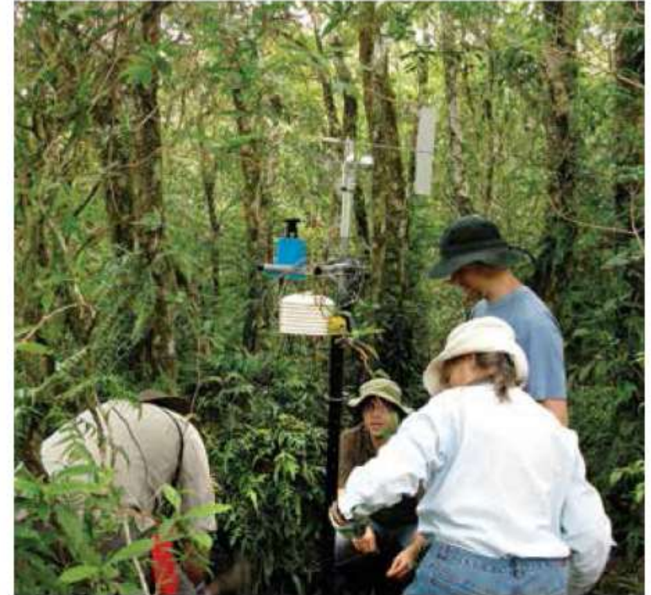
Springbrook Rainforest Project, Australia: Monitoring includes a state-of-the art, continuously operating wireless sensor network with 175 sensor nodes and 700 individual sensors providing long-term, catchment-wide micrometeorological, edaphic, and plant productivity data. A battery-powered wireless multi-media network monitors animal movements. (Case study 11) © Keith Scott
