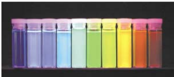
Figure 2. Ten distinguishable emission colours of ZnS-capped CdSe QDs excited with a near-UV lamp. From left to right (blue to red), the emission maxima are located at 443, 473, 481, 500, 518, 543, 565, 587, 610, and 655 nm. Reprinted by permission from Macmillan Publishers Ltd: Nature Biotech. 2001, 19, 631-635, Copyright 2001.
